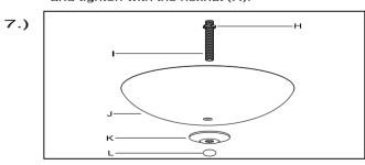
Step.7: Fit the glass shade(J) and the lid(K) onto the threaded tube(I) then tighten with the final(L).
